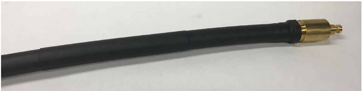
Figure 12: Heatshrink sections overlapping
